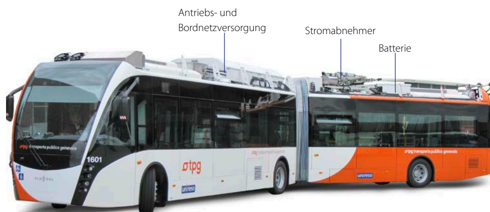
Niederflur Gelenktrolleybus ExquiCity (Kiepe Electric/Van Hool)
